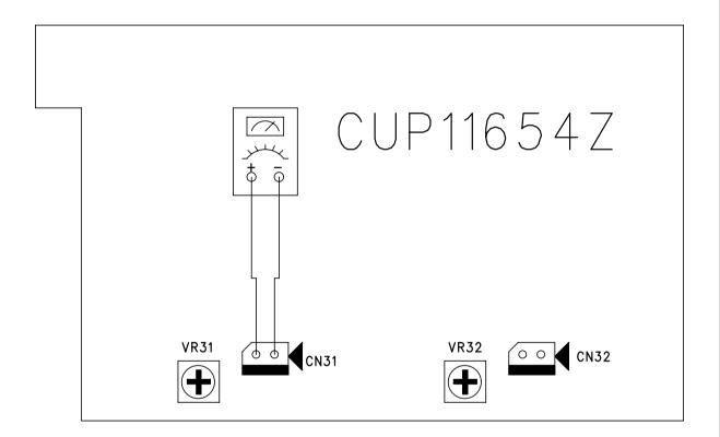
DC VOLTMETER .....Connect to CN31, CN32
