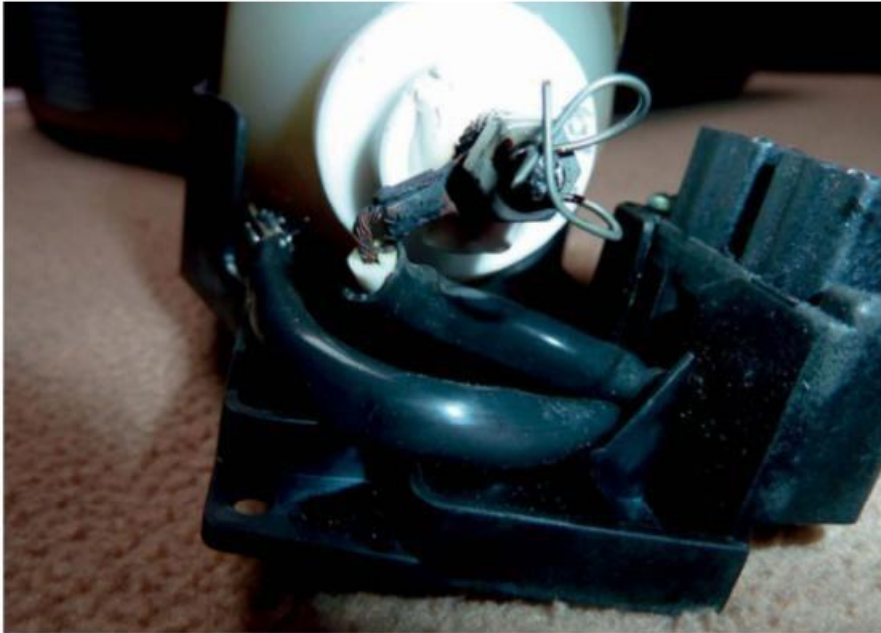
Figure 7-38. Connexion de lampe ayant surchauffé
