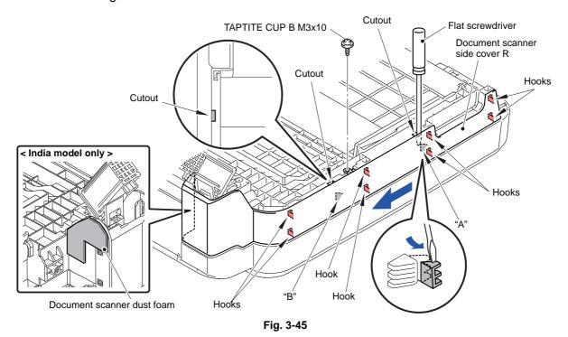
(5) Release the two Hooks and remove the Document scanner side cover R from the Document scanner unit.
