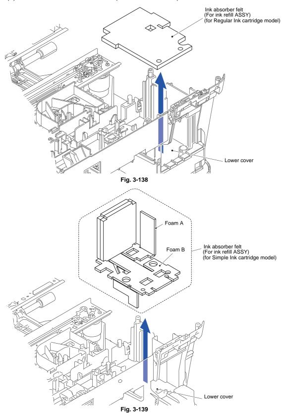
**Assembling Note:** When affixing the Foam A to the Lower cover, it must contact the top surface of the Foam B.
