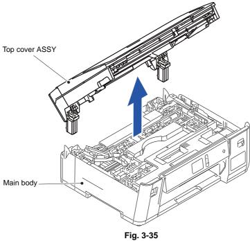
(7) Remove the three screws (TAPTITE BIND B M4x12) each from the left and right FB hinges to remove them from the Top cover ASSY.
