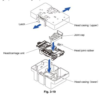
Assembling Note: Mount the Head/carriage unit, using the following steps.
