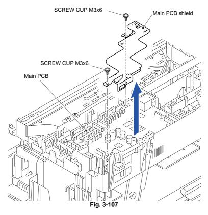
(2) Disconnect all the Connectors of the harness attached to the Main PCB harness hold L from the Main PCB.
