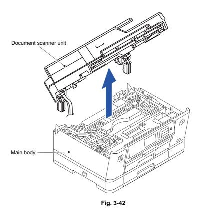
(15)Remove the three screws (TAPTITE BIND B M4x12) each from the left and right FB hinges to remove them from the Document scanner unit
