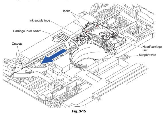
(22)Lift the Head/carriage unit from the cutouts of the CR guide rail as high as it can be removed.
