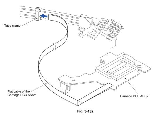
Routing of harnesses: See " Main PCB/Modem PCB", " Head/carriage unit".
