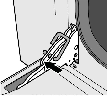
The locking pins must be fully inserted into the holes in the hinges.
