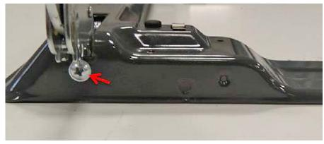
14. Unscrew the screw at the upper side of the hinge.
