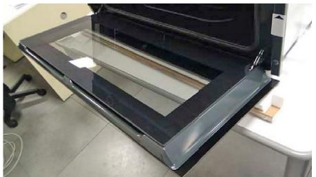
2. Lock both hinges on the left and right using the locking pin [00634525].
