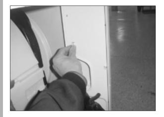
3) Remove the screw, and remove the drain pump from the lower frame.
