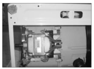
4) Remove the motor from the tub.
