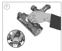
Refit the soleplate and secure locking tab.
