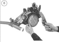
Remove the pre-filter. Ask the customer to wash if necessary (when the call has ended). Ensure pre-filter is completely dry before refitting.
