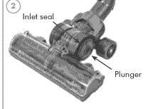
Turn machine OFF and remove turbine head. Check inlet plunger for dust/ debris. Check inlet seal for damage.
