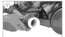
Check that the pins on the hose are not broken or bent and the connector on the inlet is not damaged.
