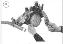
Remove the pre-filter. Ask the customer to wash if necessary (when the call has ended). Ensure pre-filter is completely dry before refitting. If machine is still not working arrange a repair.
