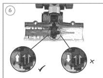
Position the brush bars back into the turbine ensuring the arrows on the brush bars are aligned with the arrow on the shaft.
