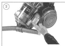
Test suction from the inlet. If suction is weak continue with checks, if strong go to step 10. Switch machine OFF.
