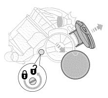
Unplug and place machine on its side for ease of access.
