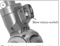
Check the stow micro-switch is not broken or obstructed.
