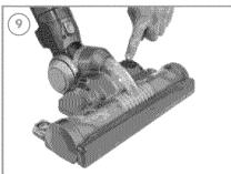
Ask the customer to refit the brush bar and end caps. Switch machine ON, press brush bar ON/OFF button and test. If customer is happy end the call. If not arrange a repair.
