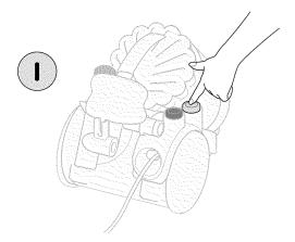
To start the machine press on/off button on the machine.
