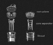
Combines Root Cyclone<sup>™</sup> technology with a core separator - an extra cyclonic stage between the outer and inner cyclones - to separate particles as small as 0.5 micron from the airflow.
