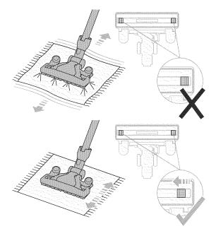
To prevent the low profile contact head from sticking to loose rugs open the bleeds on the underside.
