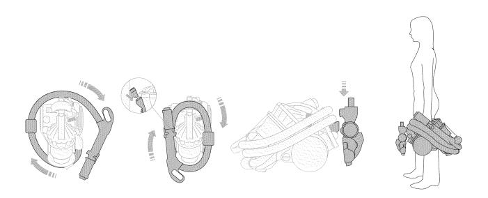
Wrap the hose around the machine and fix the wand handle in place on the side of the cyclone assembly. Place the floor tool in the parking yoke at the rear of DC23. Always carry the machine by the handle on the cyclone assembly.
