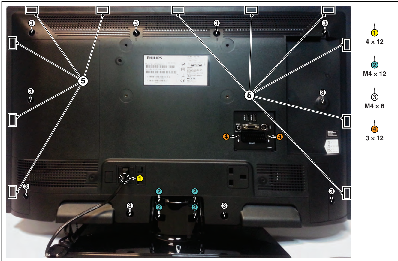
Figure 4-2 Rear cover removal
