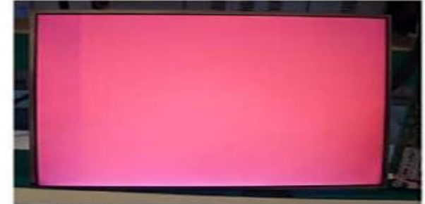
Vertical Block Source TAB IC Defect
