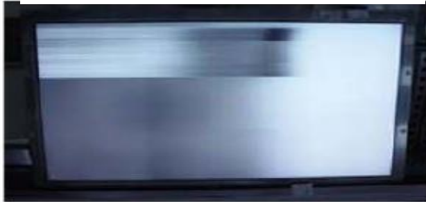
Horizontal Block Gate TAB IC Defect
