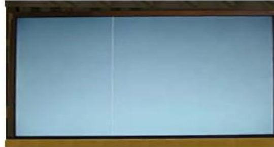
Vertical Line Source TAB IC Defect
