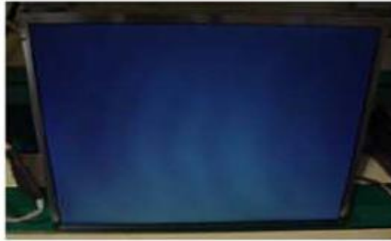
Panel Mura, Light leakage
