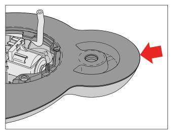
• Undo the two click connections visible on the bottom side of the appliance.
