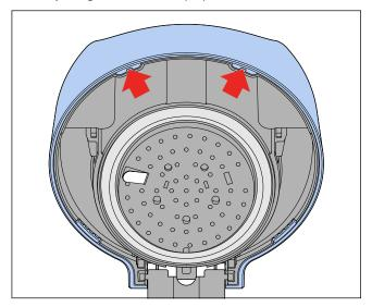
Caution, the hinge spring on the back side of the appliance may come out when the brewhead lid cover is being removed.
