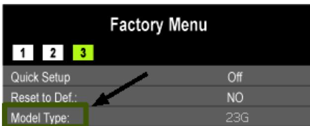
5. Select the appropriate model type by Right/Left Arrow key on the Remote.
