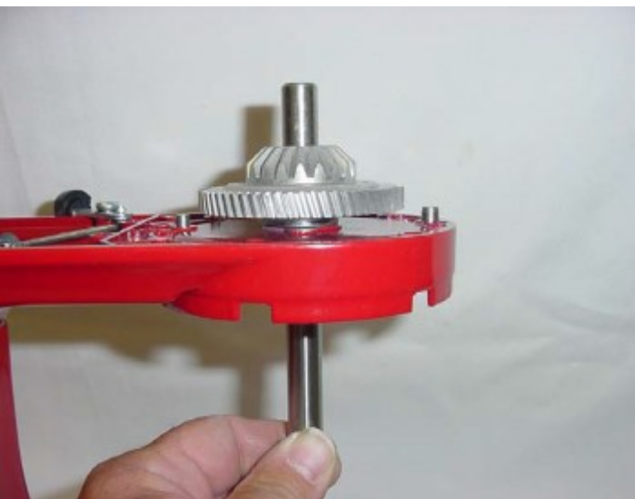
Fig. 54 Removal of vertical shaft from bottom cover.
