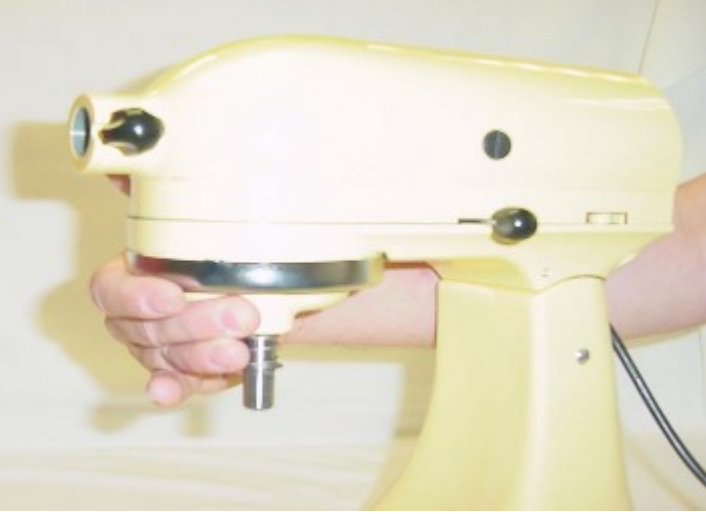
Fig. 77 Carefully let the planetary touch your finger to test speeds.
