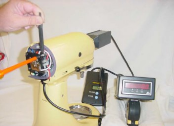
Fig. 78 Once proper speed setting has been obtained, lock the two 11/32" lock nuts.
