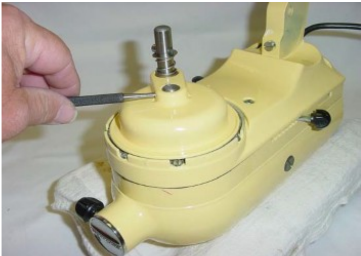
Fig. 67 A pointed punch can be used to align the holes of the shaft with the planetary.
