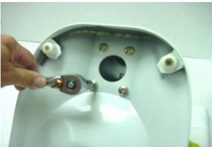
Fig. 85 Lift the column and bowl support assembly off of the bottom cover.
