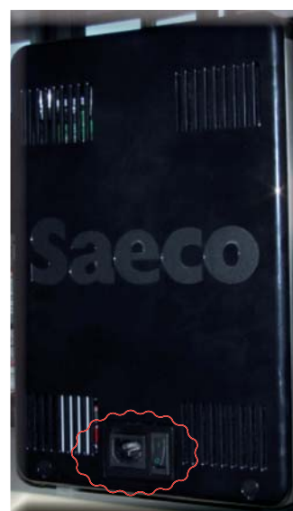
Power cable connector and main switch
