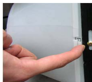
Push and pull forward lock of a bell mouth and separate bell mouth ass'y. (Be careful blade of a fan not to be deformed during disassemble)
