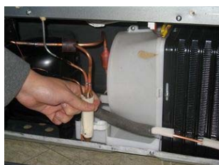
Make a space to pull out bell mouth by pushing dryer lightly which is located in front of a bell mouth to a compressor side.
