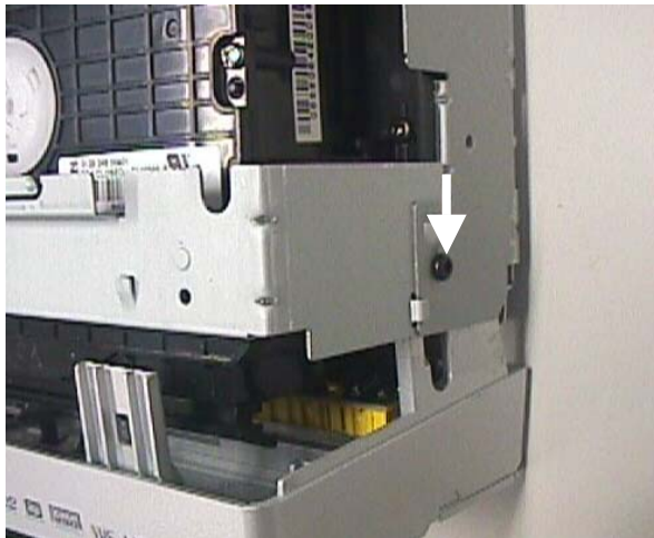
Figure 10 – Top Bracket mounting screw attached to the Frame
