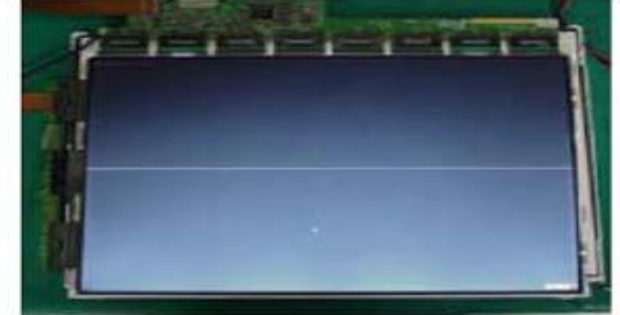
Horizontal line Gate TAB IC Defect
