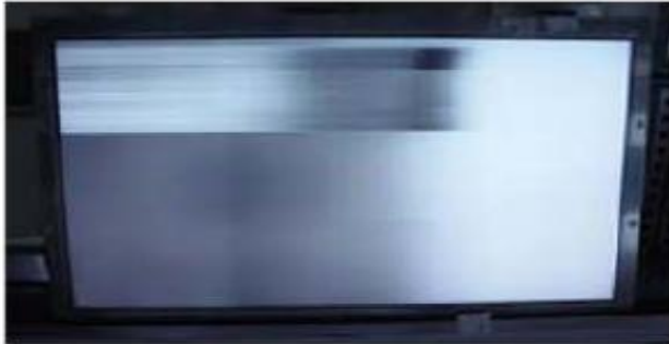
Horizontal Block Gate TAB IC Defect
