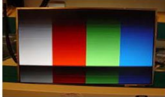
Horizontal Block Gate TAB IC Defect
