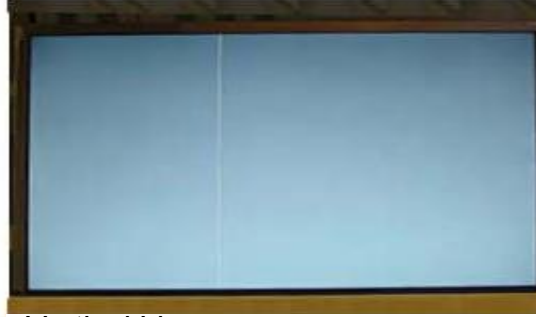
Vertical Line Source TAB IC Defect
