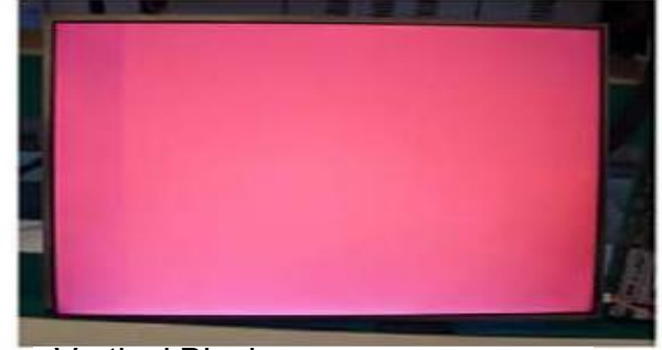
Vertical Block Source TAB IC Defect
