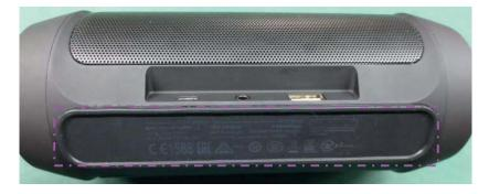
**13.** Disassemble back cover; ①Remove 4 screws by electric screw driver;
