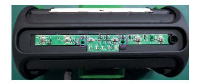
Pry up button-PCBA gently by tweezers, pull out FFC, then take out button-PCBA;
