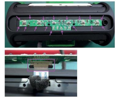
10. Remove cables; ①Pull out cables of USB PCBA, micro USB PCBA and AUX-in PCBA;
