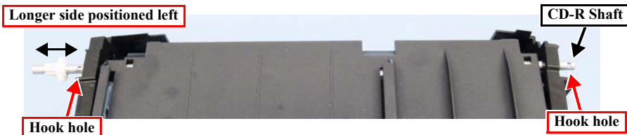
Figure 4-53. Installing the CD-R Shaft
