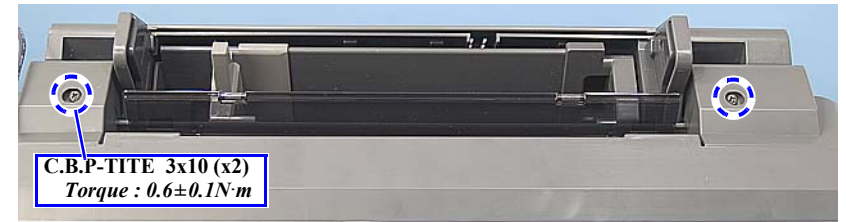
Figure 4-12. Removing the Scanner Unit
