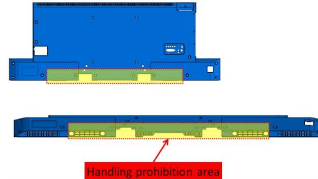
If you are going to ignore the handling prohibition area and assemble RC, when holding a middle portion, that curves then hooks will not be easily caught. And when holding SP grille portion, you will touch a speaker cone. On the other hand, when disassembling RC, you can ignore the handling prohibition area. Please refer to Appendix-1.
