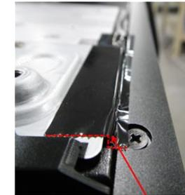
※Tape must cover the side wall of Source-Shield.
