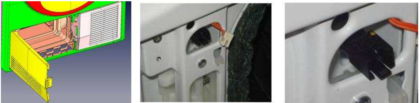
Figure 8.3. NTC located after the door filter in air suction channel
