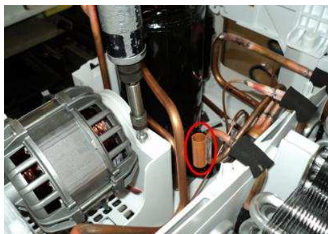
Figure 8.2. NTC located on the outlet of the condenser September' 17
