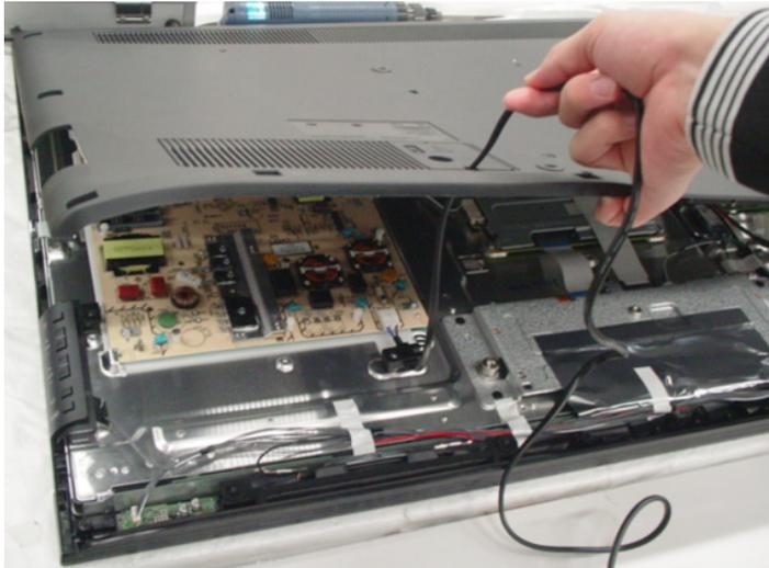
3. Disconnect the AC Power Cord to detach from Power Supply Board.
