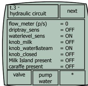
flow\_metre(p/s): Flowmetre pulses (12-17)
