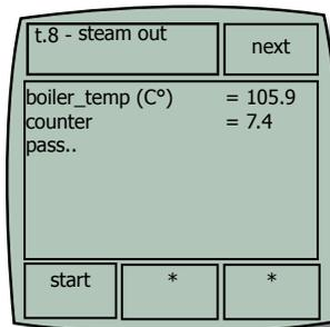
boiler\_temp (C°): heats up to approx. 110 (C°)
