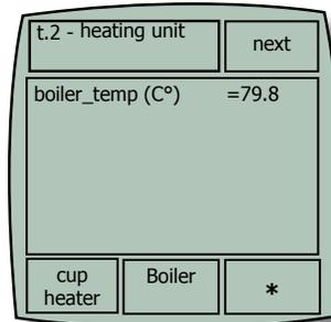
boiler\_temp (C°) Temperature recorded by the temperature sensor.
