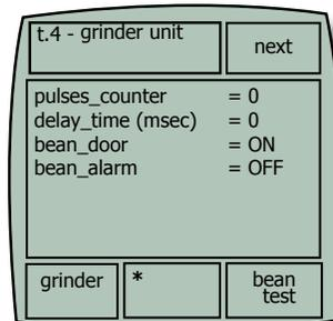
pulses\_counter: Coffee grinder pulses (Hall sensor)
