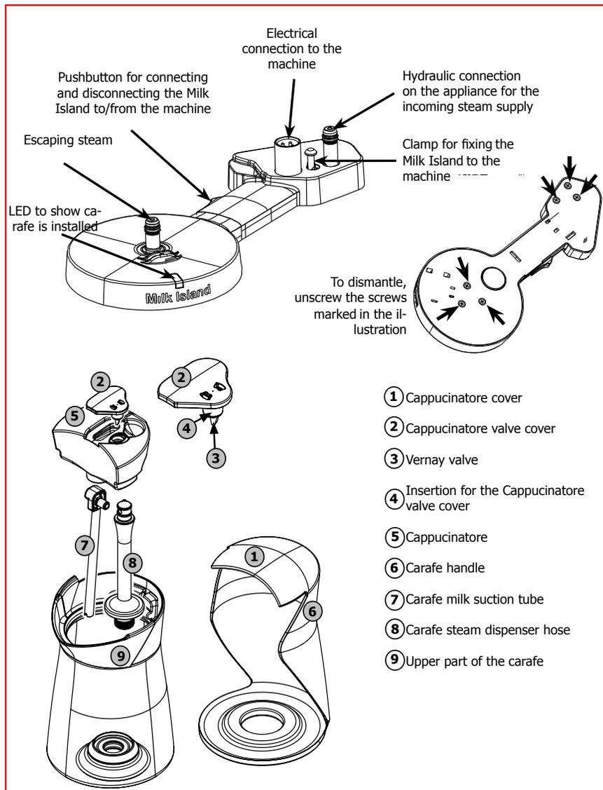
**Caution:** if the base station of the Milk Island is removed from the coffee machine, it is absolutely necessary to apply the lock on the bottom of the machine!
