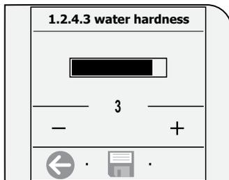
Carry out the settings with the +/- keys and save with the
