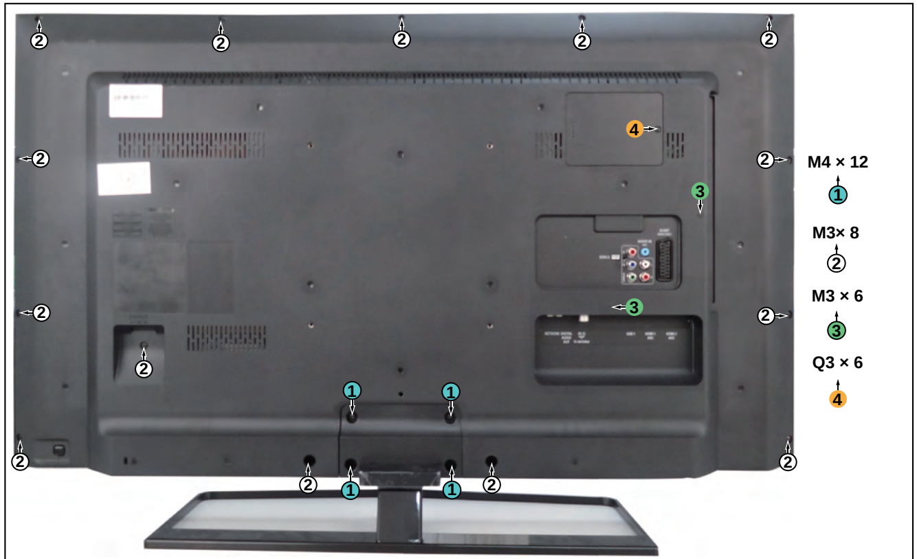
Figure 4-16 Rear cover removal[1]
