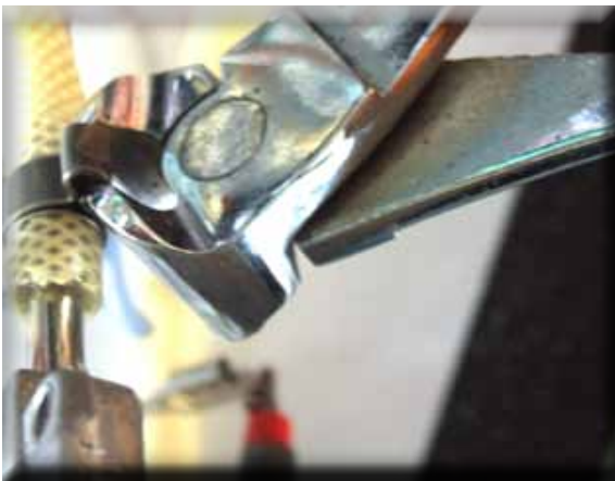
To remove the clamp use appropriate pliers, as shown in the picture
