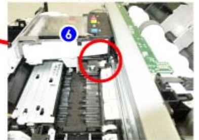
6. Carriage encoder sensor
