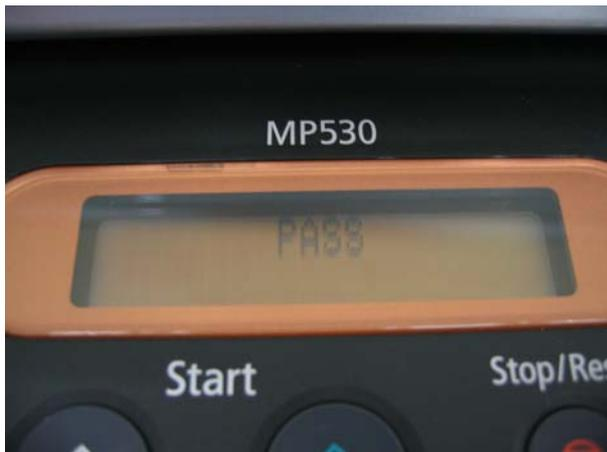
5) Open the scanning unit (printer cover), then press the ON/OFF button to complete Button and LCD test and return to the service mode menu selection.
