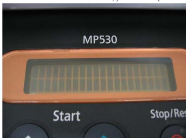
2) Press the Stop/Reset button again, then the following screen is displayed.
