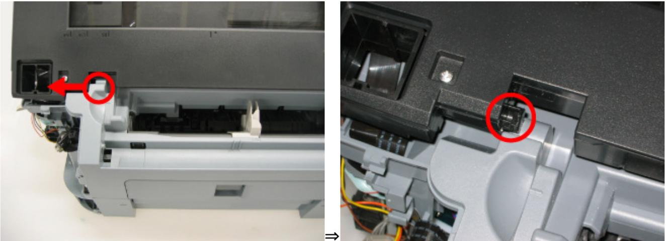
g) Slide the scanner to the arrow-indicated direction to release the hook, then remove the Scanner Unit.
