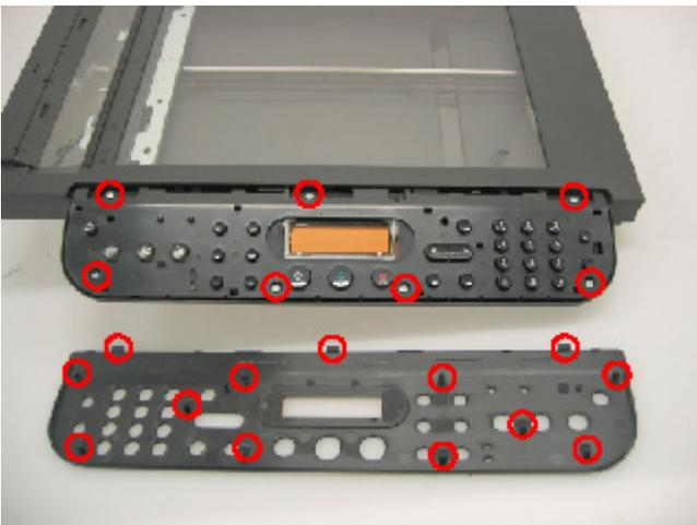
b) Remove the seven screws, then disconnect the flexible cable and connector.
