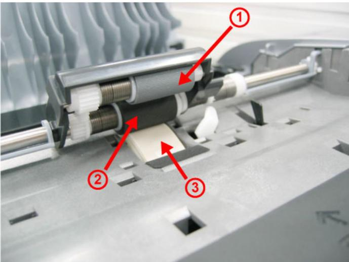
**(19) Removal of the parts inside the ADF Unit**
