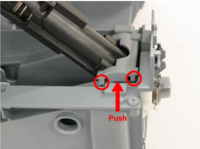
d) Pull the right and left metal parts to the arrow-indicated directions, then disengage the Scanner Stop Arm Unit by lifting it.
