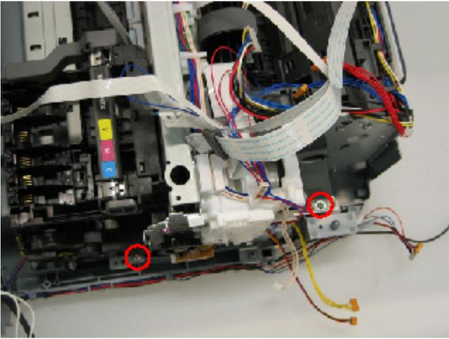
**(16) Operation Panel Unit / LCD Unit removal**
