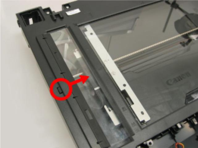
**(18) Document Feed Roller, Separation Roller, and Separation Tab cleaning**
