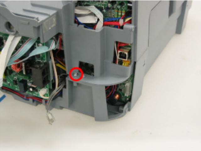
c) Disconnect the connector for the solenoid.
