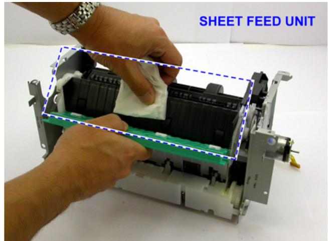
\*3: How to make and set the ASF sub-roller cleaning sheet:
