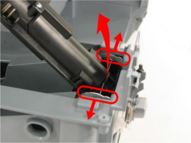
e) Remove the two screws from the Damper Joint.
