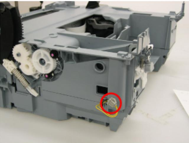
d) Disconnect the connector of the Scanner Open Switch.
