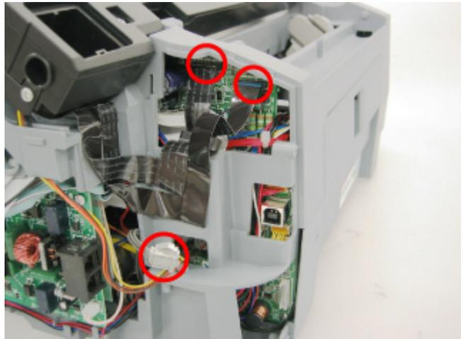
c) Push the Scanner Lock to release the two hooks, then lift it.
