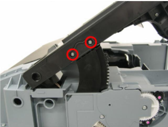
f) Slide the scanner unit toward the arrow-indicated direction and lift the unit; the hook will be released.
