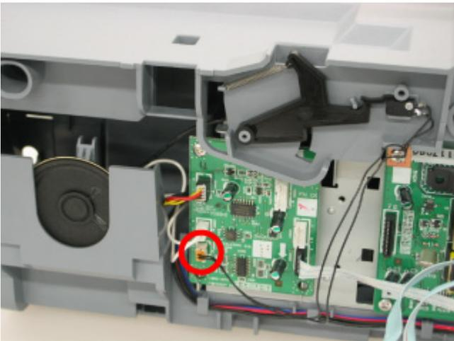
e) Release the two hooks using a flat-blade screwdriver, etc., then lift up the Main Case.
