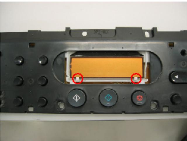
**(17) DF Guide Sheet Holder / DF Guide Sheet removal**
