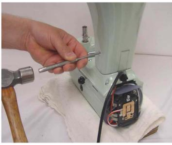
Fig. 4 A drift punch and hammer is used to drive out the hinge pin.
