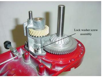
Fig. 59 Secure the three lock washer screw assemblies into the bottom cover.
