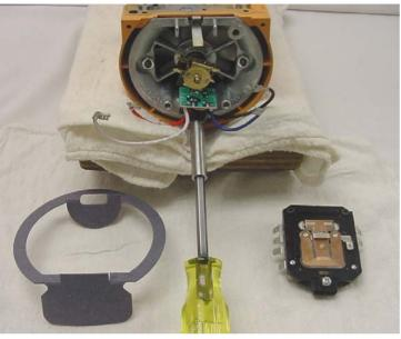
Fig. 48 The triac is shown being secured to the bearing bracket.
