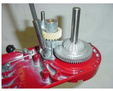
Fig. 52 Worm gear bracket bearing and pin assembly.
