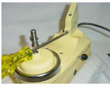
Fig. 69 The adjusting screw has a nylon insert and should not be loose in the threads.
