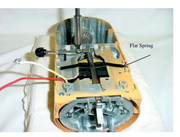
Fig. 24 The pivot screw and tension washer are removed with a phillips screwdriver.
