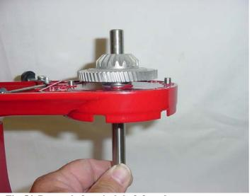
Fig. 54 Removal of vertical shaft from bottom cover.
