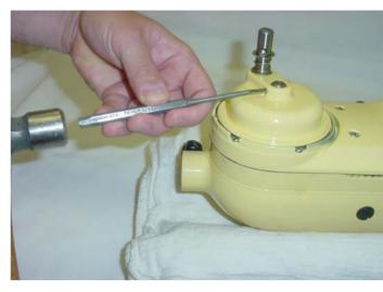
Fig. 68 Carefully drive the groove pin into the shaft of the planetary.
