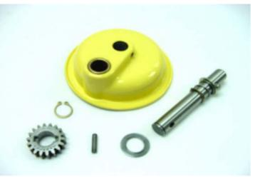
Fig. 66 The planetary components are shown disassembled.
