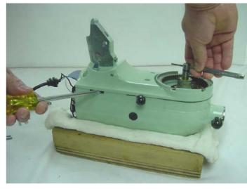
Fig. 12 While lifting up on the center shaft, use a screw driver to gently pry the bottom cover from the housing.
