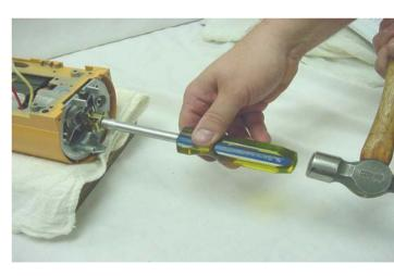
Fig. 47 Using a 3/8" nut driver to seat the governor. Tap gently. Never drive directly against governor ball.
