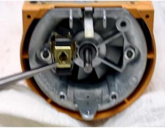
Fig. 22 Governor shown removed from the shaft of the motor.
