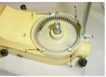
Fig. 62 Tighten the five special screws evenly to 18-20 in. lbs.. torque using the sequence shown.
