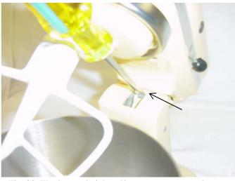
Fig. 83 The beater height adjustment screw used to set the 1/16" clearance between the bowl and beater.
