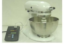
**KitchenAid stand mixer shown with a digital wattmeter** If the wattmeter shows up to 135 watts, going from stir to #10 speed, the mixer is in good condition.
