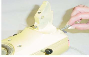
**Fig. 63 Secure the four fillister head screws.** The bearing is an integral part of the planetary. Hold the agitator shaft firmly and remove the pinion retaining clip (Fig. 64).
