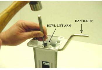
Fig. 89 Drive out the roll pin to remove the bowl lift arm.
