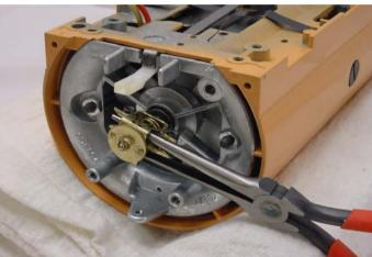
Fig. 21 Needle nose plier used to pry governor off the motor shaft.
