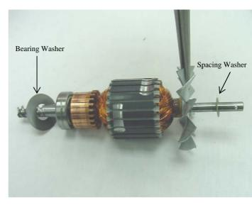
Fig. 38 Check the blades of the armature ventilating fan and straighten if bent.
