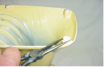
Fig. 71 The pedestal feet should be replaced on older mixers.
