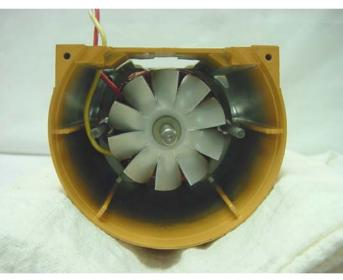
Fig. 39 Locating the armature into the gearcase-motor housing.
