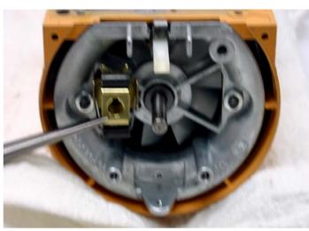
Fig. 45 The governor shown before being placed on the motor shaft.
