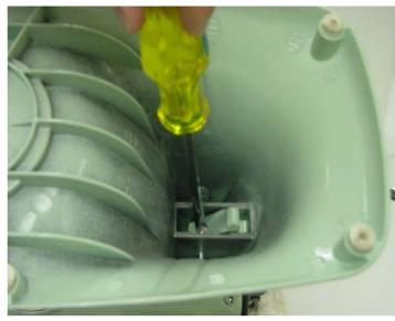
Fig. 3 Loosen the hinge pin setscrew to remove the pedestal from the bottomcover.
