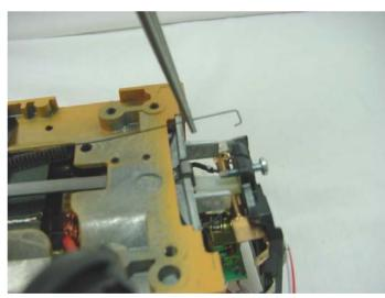
Fig. 17 Unhook the control board spring.
