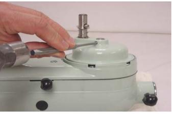
Fig. 6 Removal of the groove pin that holds the planetary to the vertical center shaft
