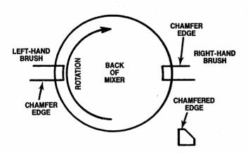
Fig. 34 The orientation of the brush holder inserts viewing from the rear of the motor housing.
