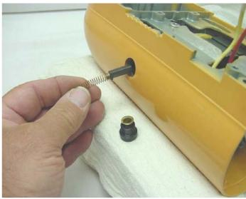
Fig. 29 the brush holder caps are loosened to access brushes for removal. Make sure to mark orientation.
