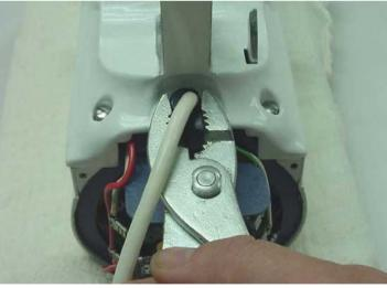
Fig. 9 Removal of Heyco strain relief using pliers.
