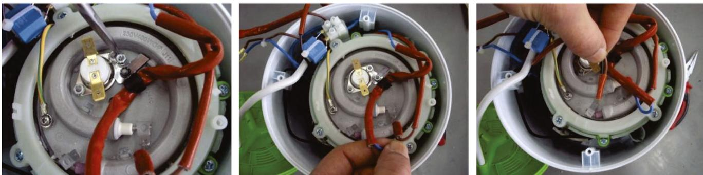
5th operation Attaching the heating plate cable and thermostat cables
