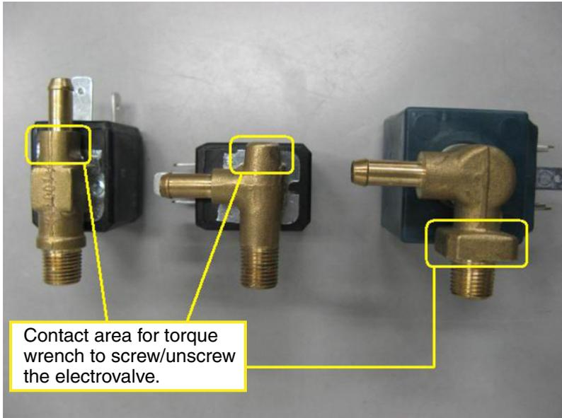
CAUTION #2: Ensure torque wrench jaw does not contact the solenoid body.
